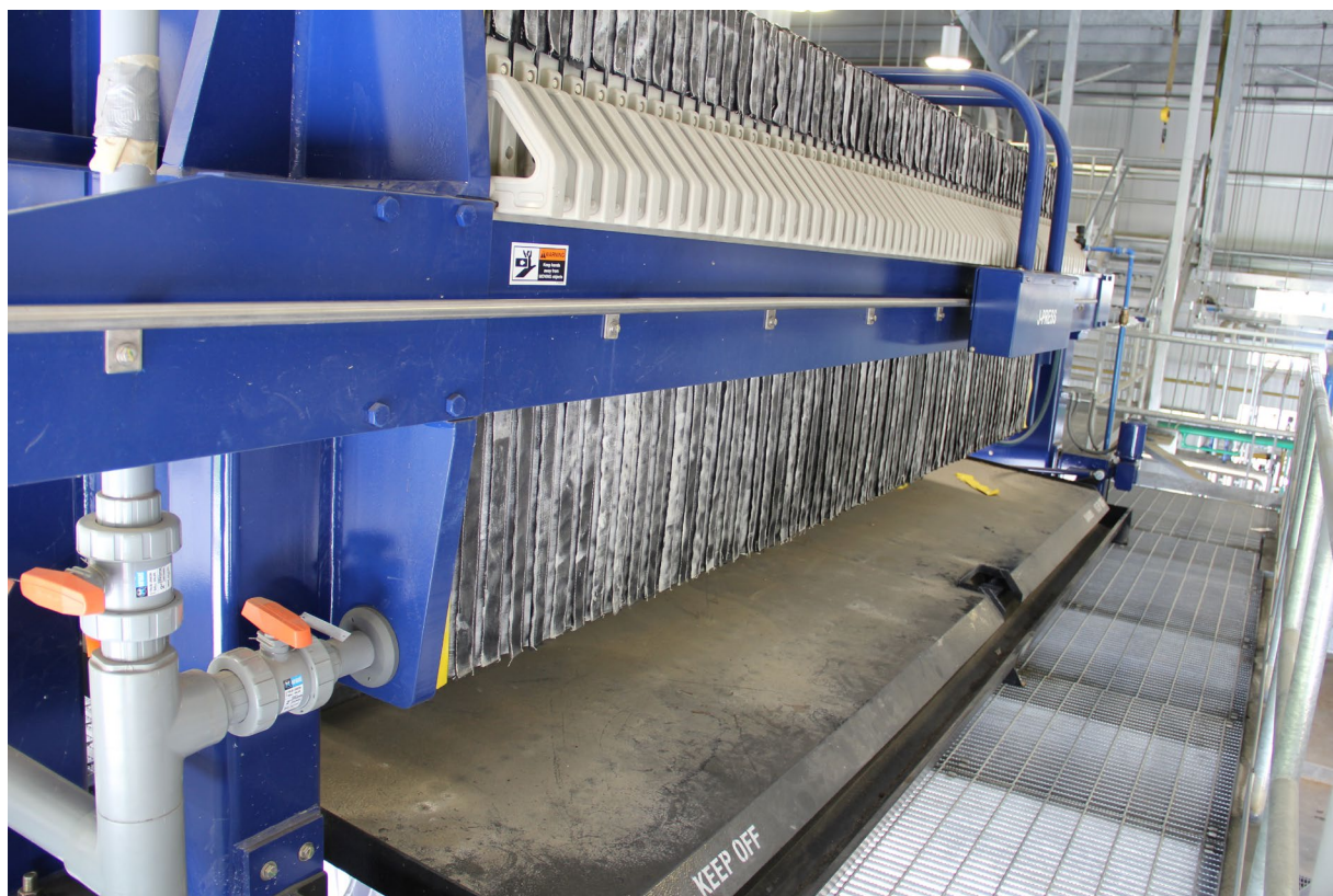
CLEANING UP: The water treatment facility has a filter press to dewater sludge in the wastewater process.
