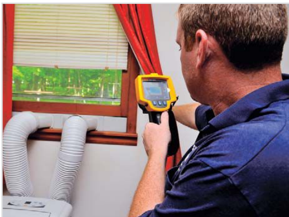
An energy efficiency specialist checks for air leaks and the effectiveness of a window's seal.
